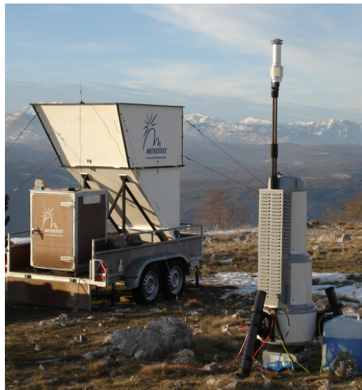
Figure 1: The measurement site Maligrad with the SODAR (left) and the ZephIR LIDAR (right).
