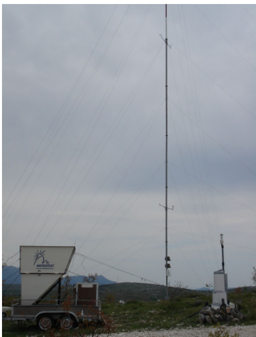
Fig. 3: Picture of SODAR (left), 50 m mast and LIDAR (right) at Rudine facing south-east.
