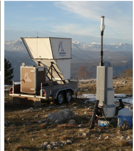
Fig. 1: The measurement site Maligrad with SODAR (left) and ZephIR-LIDAR (right).
